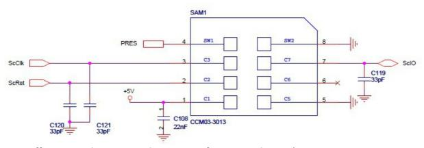
(C1 pin off SAM1 can be connected to 3V3OUT for 3,3V application)
