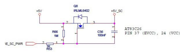
AT83C26's oscillation circuit (U5's pin 1) can be disabled by inverting H663's E\_SC\_PWR using an open collector inverter gate.
