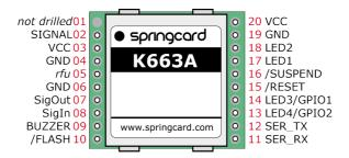
$<sup>^{1}</sup>$  Note that in a most situations, K663A could be used as drop-in replacement for earlier K531 or K632.
