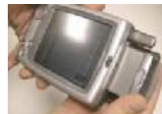
For other Pocket PC, strongly hold the module and pull in the axis of the CompactFlash port
