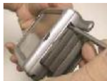
For SX45 pocket PC, press on the auto-extractor button with the pen.
