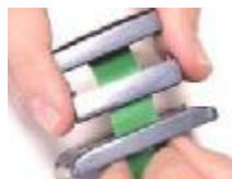
Extract the CompactFlash part from the brace
