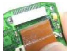
Pull down carefully while holding the PCB in the other hand
