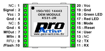
Module is powered by Vcc = 5V.
