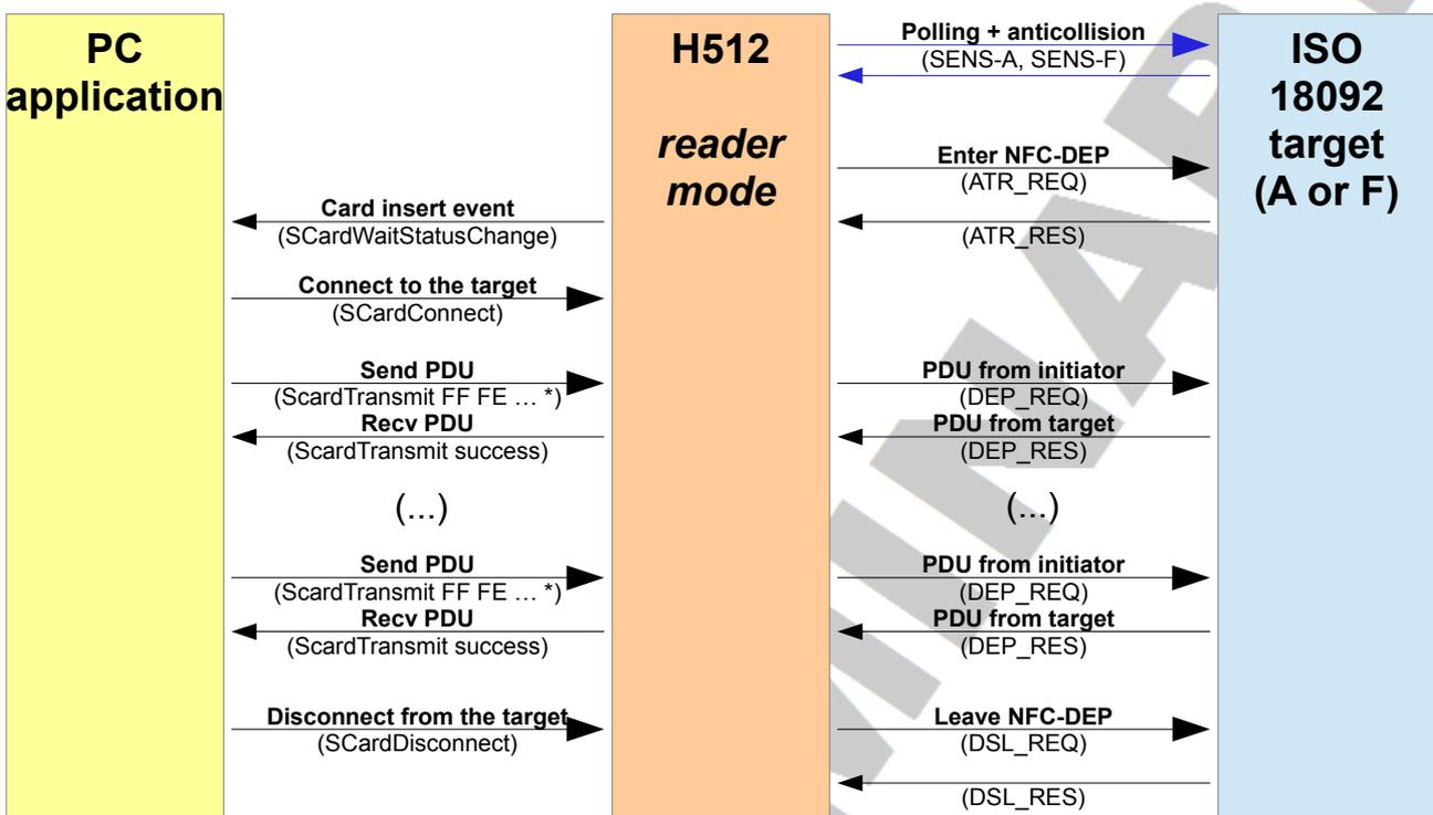
\* The PDU must be ENCAPSULATED if it doesn't meet ISO 7816-4 constraints.
