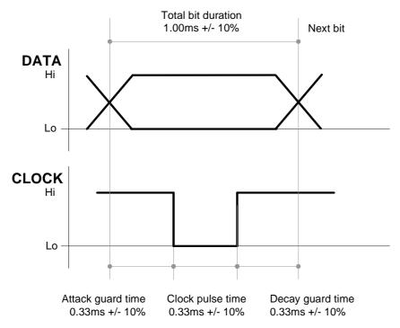
It is better that the controller triggers on the falling edge of the clock or on the low level, and not on the rising edge.
