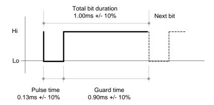
It is better that the controller triggers on the falling edge of the signal or on the low level, and not on the rising edge.
