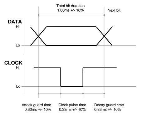
It is better that the controller triggers on the falling edge of the clock or on the low level, and not on the rising edge.
