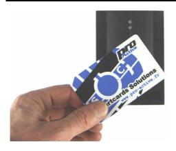
IWM-K632-SU is an highly customizable wall-mount contactless reader. It reads virtually any kind of ISO/IEC 14443 proximity cards, and ISO/IEC 15693 vicinity tags or transponders.
