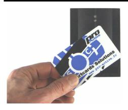
IWM-K632-WD is an highly customizable wall-mount contactless reader. It reads virtually any kind of ISO/IEC 14443 proximity cards, and ISO/IEC 15693 vicinity tags or transponders.
