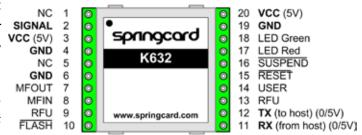
NB: the K632 needs an external antenna to operate.
