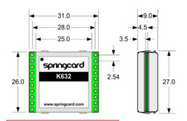
Unit = millimeters Tolerance ± 0.1 on all dimensions
