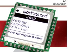
H632 is a reader/writer module compliant with 13.56MHz RFID and NFC standards (ISO 14443, ISO 15693) also able to drive up 5 contact smartcards. Its small footprint and single 5V power supply make H632 the ultimate interface to be integrated in validators, ATM or vending machines, cash registers, ...
