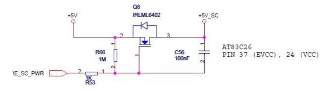
**AT83C26**'s 5V power supply is driven by **H663**'s E\_SC\_PWR pin (#15).
