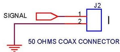
When the distance between the module and the antenna is short enough (< 50mm), an unshielded twisted pair, or copper lines on the PCB could be used instead of the coaxial cable.
