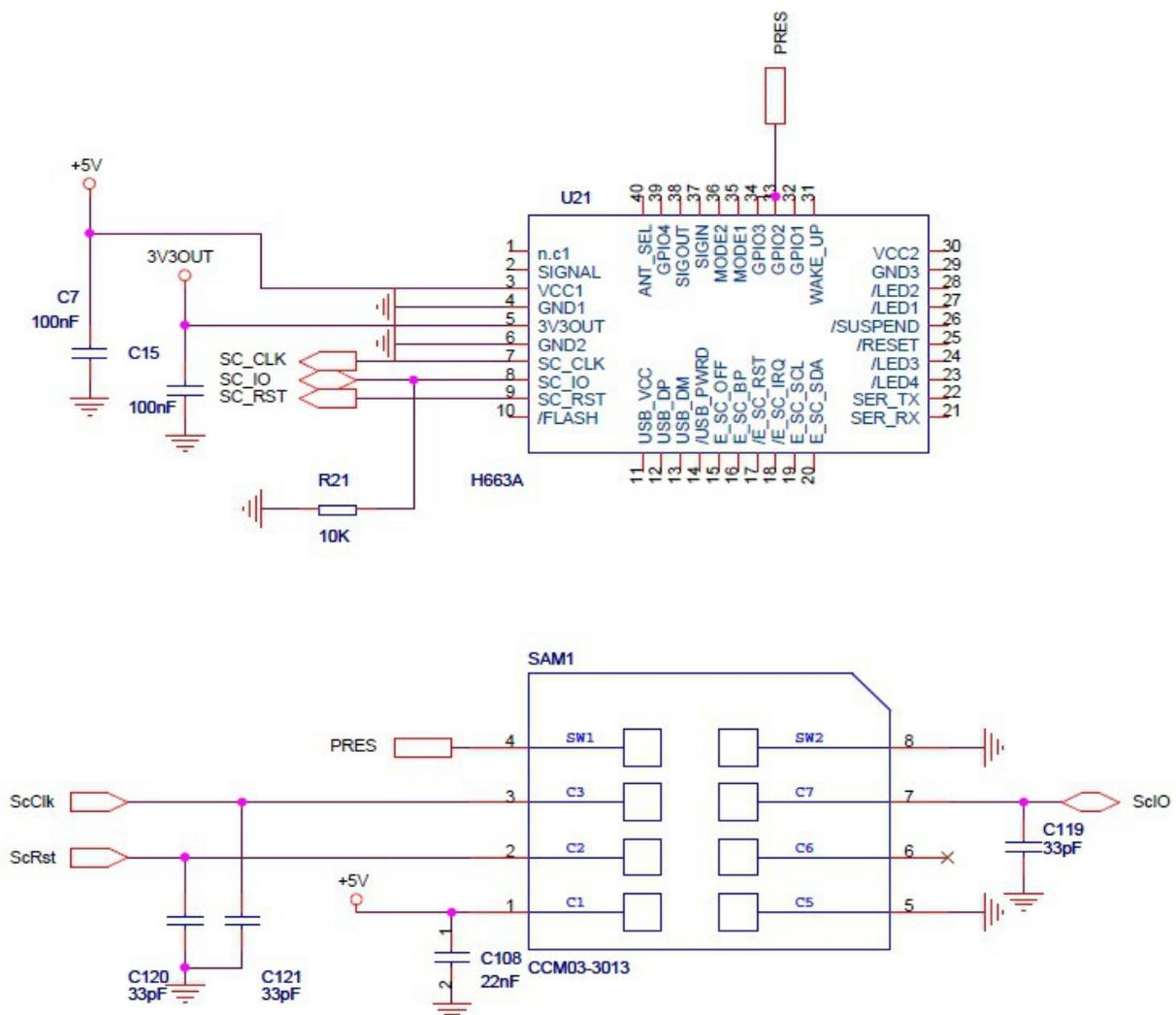
(C1 pin off SAM1 can be connected to 3V3OUT for 3,3V application)
