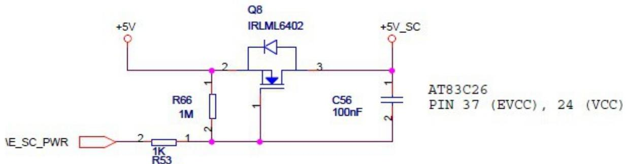
AT83C26's oscillation circuit (U5's pin 1) can be disabled by inverting H663's E\_SC\_PWR using an open collector inverter gate.
