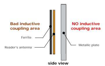
**Example 3**: metallic plate is behind the ferrite and is distant enough (L) from both ferrite and antenna. YES!
