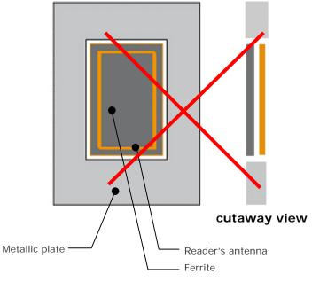
**Example 5**: Both ferrite and antenna are positioned inside a rectangular hole of the metallic plate which is wide and high enough to not interfere with the magnetic field lines of the antenna. YES!
