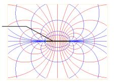
The reader's antenna generates a magnetic field that creates an inductive coupling with the card/tag's antenna present in the field. This **power transfer** is the basis of the HF communication between contactless readers and cards/tags. As a consequence, care should be taken in order to optimize this coupling.
