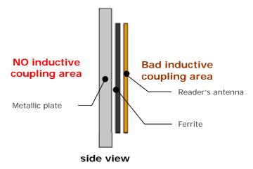
Example 2: metallic plate is in front of the antenna and too close to both ferrite & antenna. NO!
