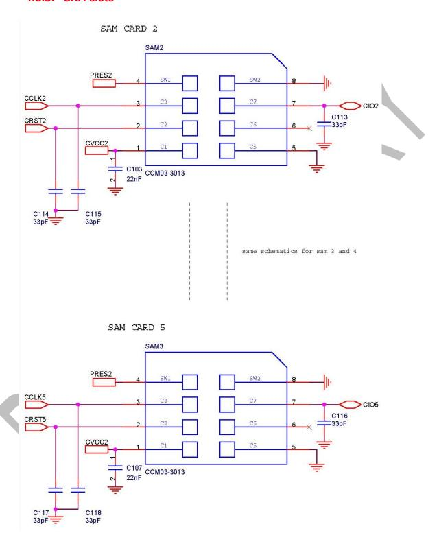
$1^{\rm st}$  SAM slot (SAM CARD 2) has its own card presence input within the AT83C26 (PRES2). Presence of the card in the other slots (SAM CARD 3 to SAM CARD 5) is monitored through a PCF8574 component (I2C I/O interface).
