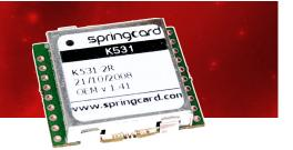
K531 is an ISO/IEC 14443 contactless reader/writer module for OEM integration
