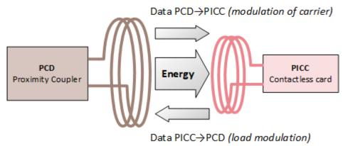
The magnetic field emitted by the coupler not only provides a power supply to the card, but is also carrying data in both directions: The coupler modulates its carrier to send its orders, the card uses load-modulation to answer.
