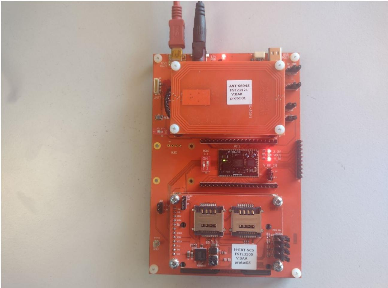
Illustration 1: M519-SRK connected to the PC through its FTDI USB to Serial bridge
