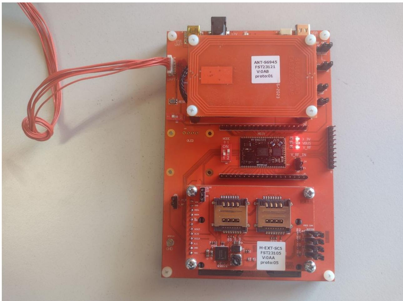
*Illustration 2: M519-SRK connected and powered through its JST 8 connector*
