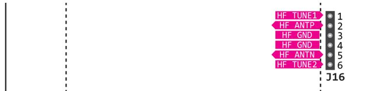
Illustration 5: Pinout on header J16 (interface to NFC/RFID HF antenna)
