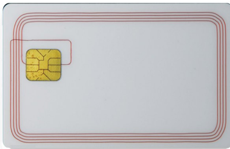
Illustration 9: A first-generation's dual-access card, featuring a copper coil welded behind the ISO/IEC 7816 module
