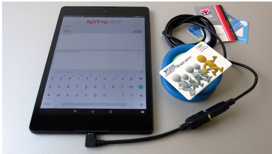
Illustration 22: A Nexus 9 Android Tablet with a Prox'N'Roll PC/SC HSP
