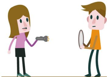
In **passive RFID**: the target does not have an emitter. In order to make itself “heard”, it does not have any other choice than alter the interviewer wave. This technique is called backscattering or retro-modulation. For example, a pilot who would stick his arm out of the cockpit window and wave a big flag reflecting waves, would produce on the radar screen a “spot” blinking in an unusual manner. It could be recognized by the base station, without issuing any wave !
